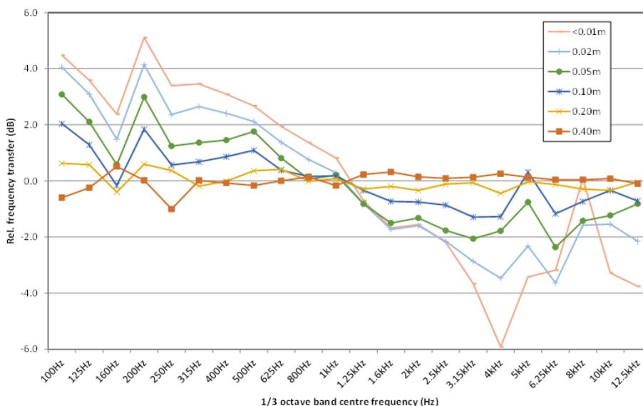
Figure 7. Frequency transfer function of the Bedrock BTB65 Talkbox as a function of distance (SPL 60 dB(A) at 1 meter distance).
