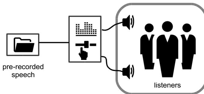
Figure 4. Schematic representation of a PA/VA system that uses pre-recorded messages. A talkbox is not needed.
