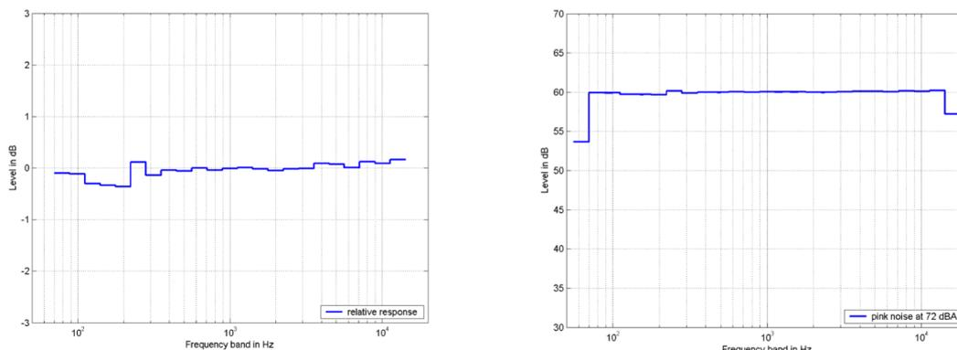
Figure 6. Typical example of the (corrected) frequency transfer function of a Bedrock BTB65 talkbox (left), meeting the specifications as defined above. The right panel shows the spectrum when playing back pink noise at a level of 72 dB(A)
