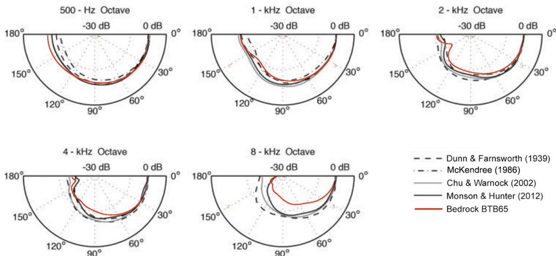
Figure 8. Directivity of the Bedrock BTB65 in the horizontal plane (red curve), compared with the directivity of human speech according to 4 different studies (after [6]). Data for lower octave bands have been omitted, since the BTB65 as well as human talkers show near-perfect omnidirectional behaviour.
