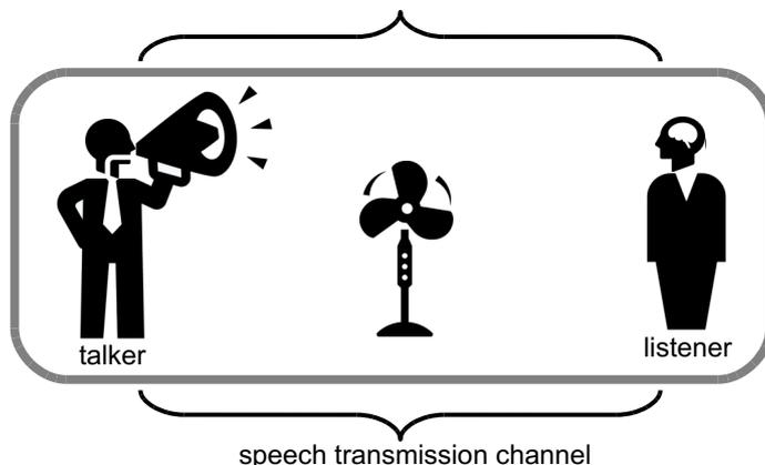
Figure 3. Schematic representation of the definition of a speech transmission channel. The channel comprises everything between the talker and listener that influences intelligibility, including noise sources and the acoustics of the environment, except for the talker and listener themselves.
