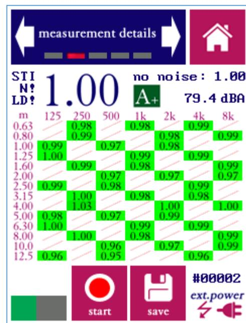
Figure 5. Full STI implementation on the Bedrock SMxx, while measuring. The analyser is synchronized and in the second stage of the signal.
