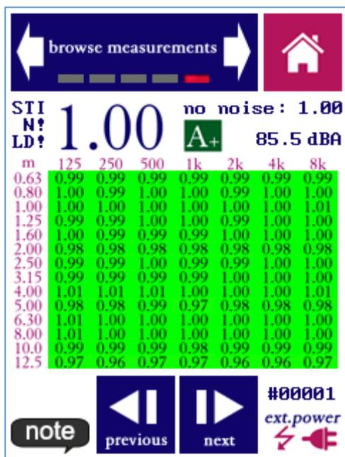
Figure 6. The full STI measurement has completed (in this case, for a perfect transmission channel). The MTF matrix is completely filled.
