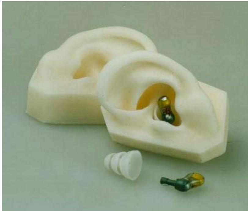
Figure 4. Wireless Communications Earplug receivers (in an artificial ear and separately).
