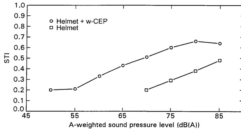
Figure 8. STI as a function of A-weighted intercom speech level at the tympanic membrane, in representative ambient noise (Chinook cargo compartment, 111 dB(A))
