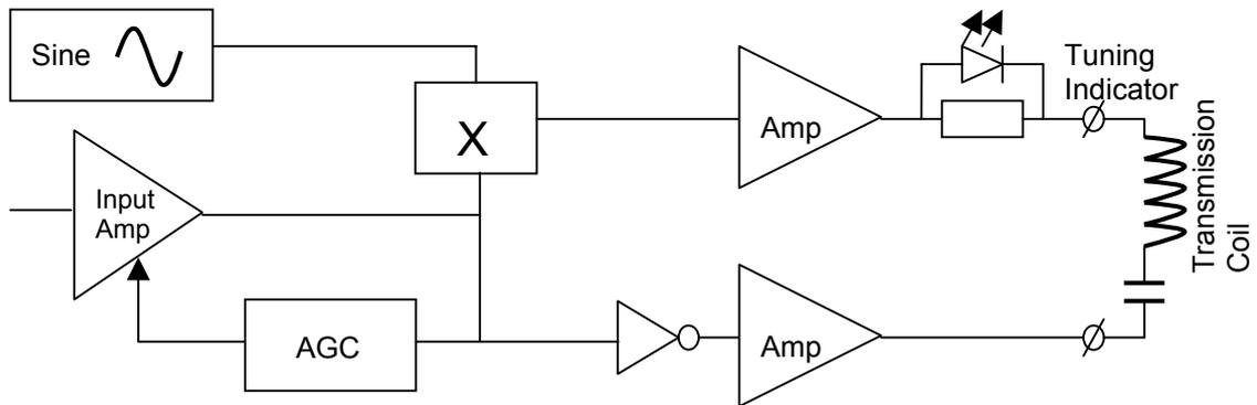
Figure 5. Simplified block diagram of the transmitter.
