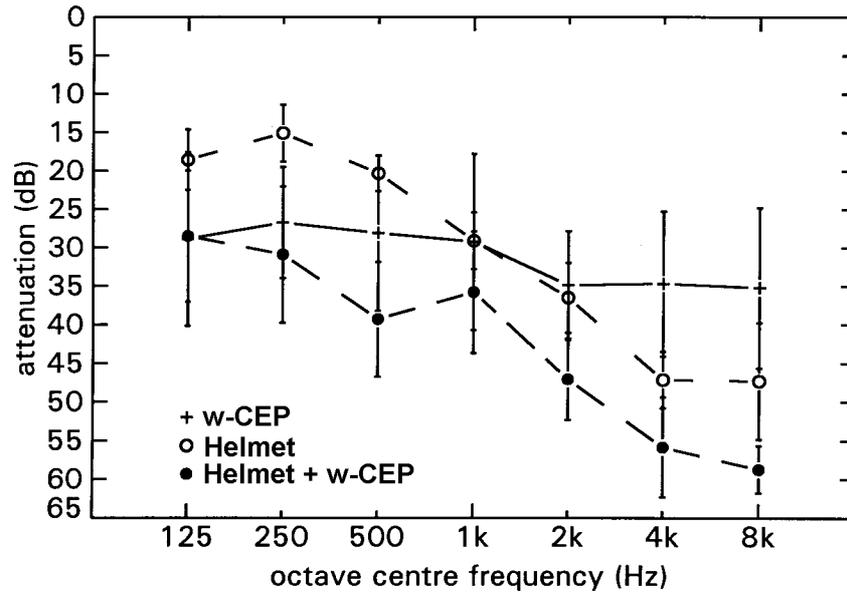
Figure 6. Sound attenuation according to ISO 4869-1 (average and standard deviation, 16 subjects) for the wireless CEP earplugs, a common type of helmet and the combination of helmet and earplugs.
