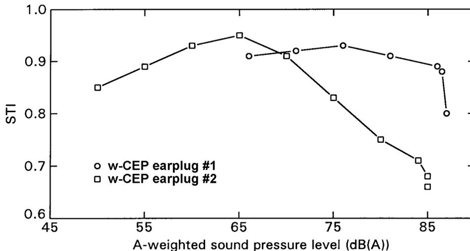
Figure 7. STI as a function of A-weighted sound pressure level *of the intercom speech* at the ear, for two prototype versions of the w-CEP earplugs.
