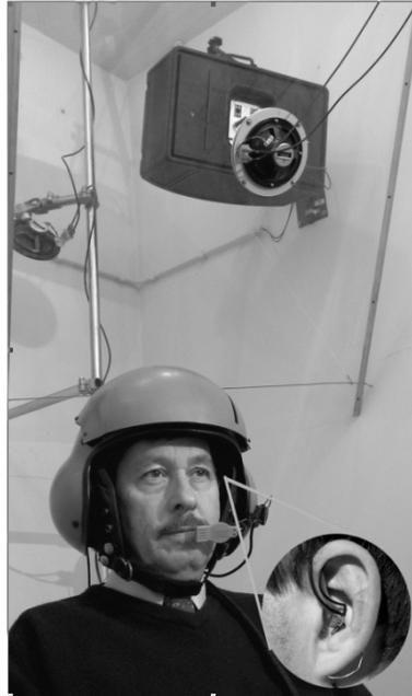
Figure 21. Subject positioned in a high-noise room and the mounting of the electret microphone near the entrance of the ear canal.
